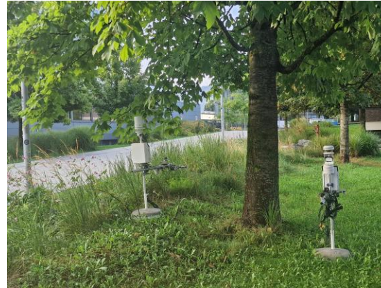
Atmos 41 Weatherstation 12 Parameters
