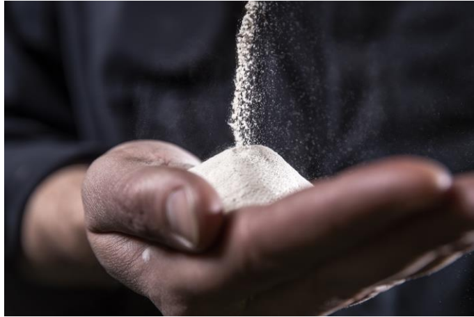
Figure 20. Apatite concentrate produced from mine tailings during ReeMAP pilot phase.
