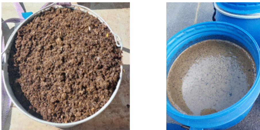
Figure 38. Separated solid (left) and liquid (right) fractions of digestate
