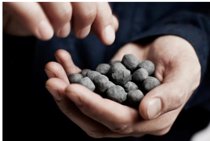
Figure 19. LKAB iron ore pellets, each with ~67 % iron concentration.
