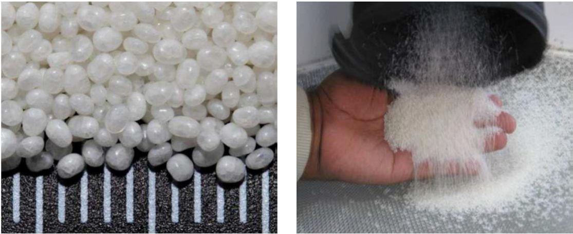
Figure 24. Struvite produced using the Ostara Technology.
