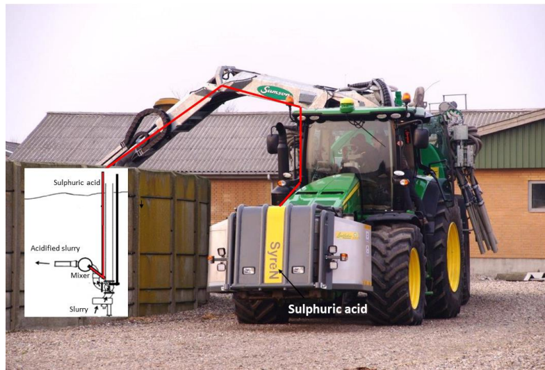
Figure 14. Acidification of the slurry.
