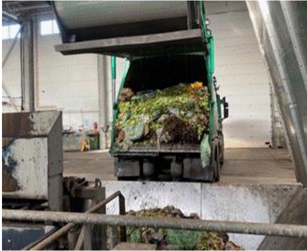
Figure 36. Separately collected bio-waste being unloaded into the reception bin (left), grocery store waste awaiting pre-treatment at EcoBio before entering the fermenters (right).
