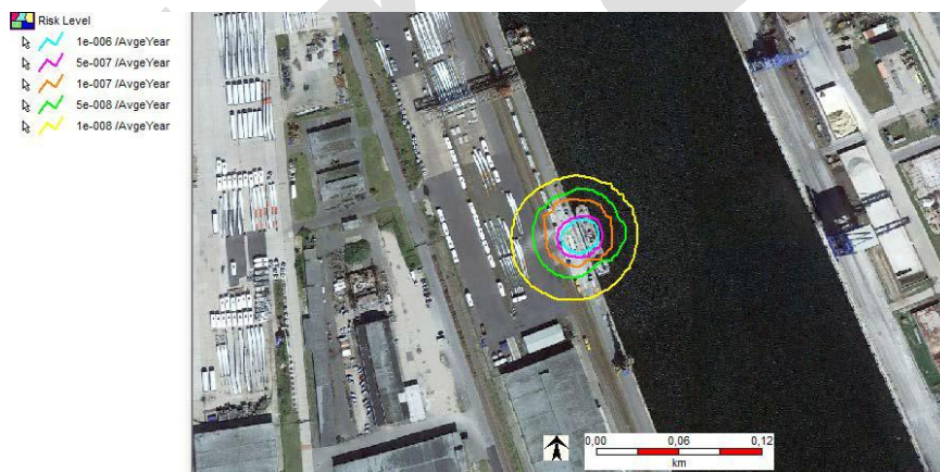
Figure 3-6 Risk contours from SAFETI for a bunker site with a given set of release scenarios
