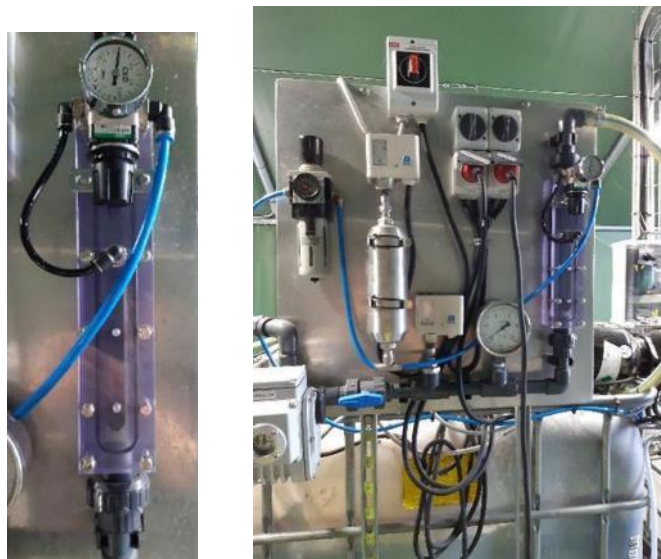
Figure 9. Nanobubble generator and setup
