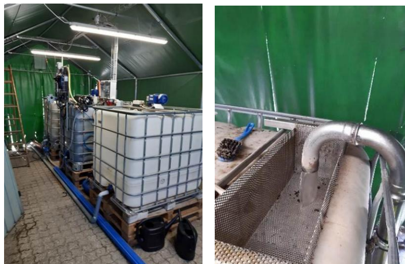
Figure 8. Pilot plant to test nano bubble technology.
