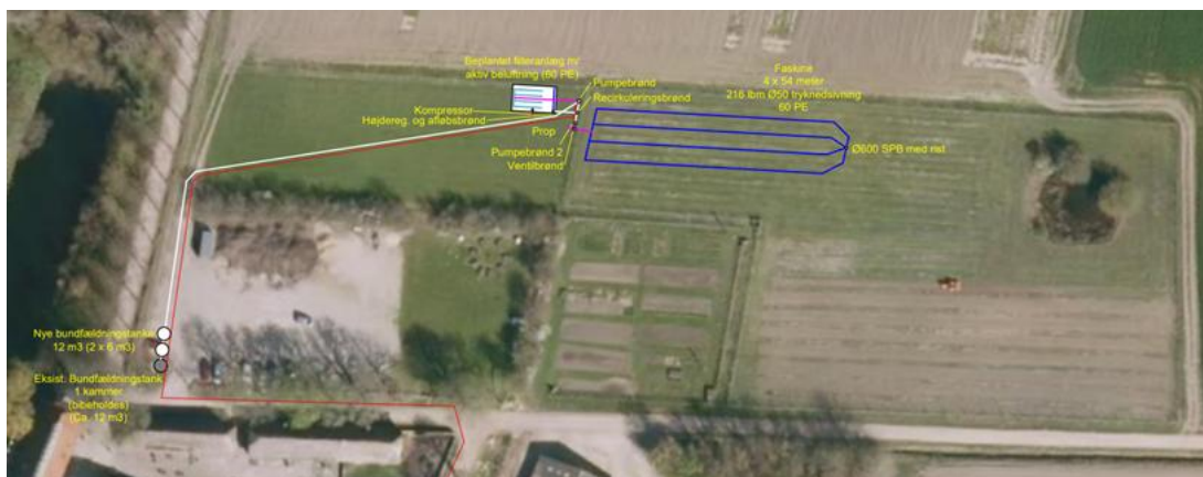
Figure 13. Skovgaard Gods with the location of the intensified constructed wetland and a zoom of the area
