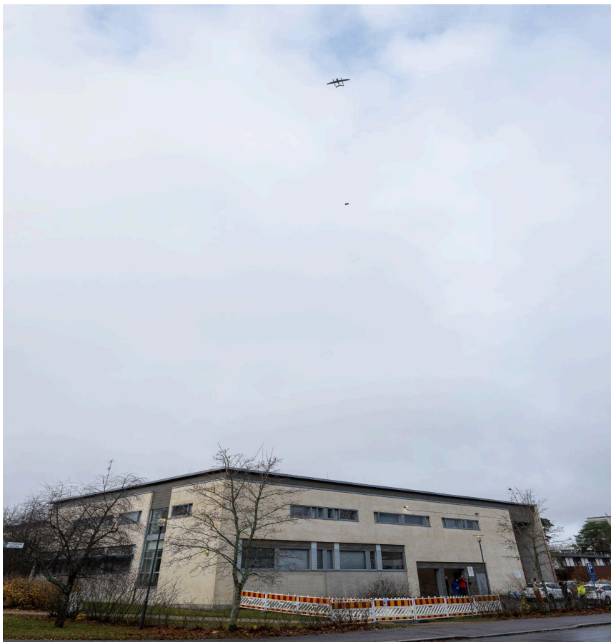
Image 22 & 23: The drone hovered at an altitude of 60 meters before lowering a shoebox-sized box via a cable on a specified 4x4-meter designated landing site right next to the health station's logistics entrance.
