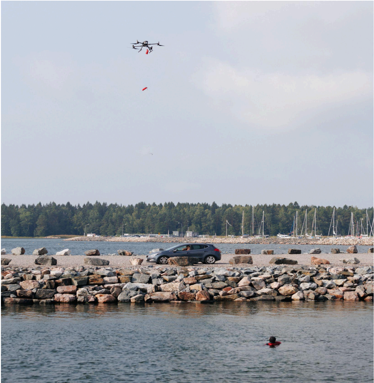
Image 20: The drone successfully brought the floating device down and close enough to the Helsinki City Rescue Department staff member who was simulating a person in distress.
