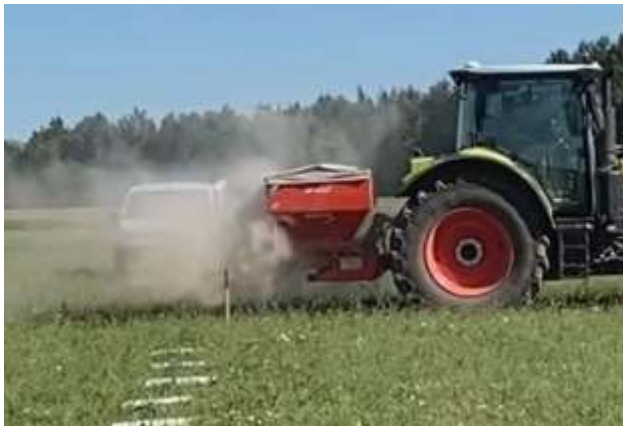
Figure 3. Generation of excessive dust during the spreading of mechanically weak fertiliser granules using a field spreader (Photo by Tamm, Kalvi , 2023).
