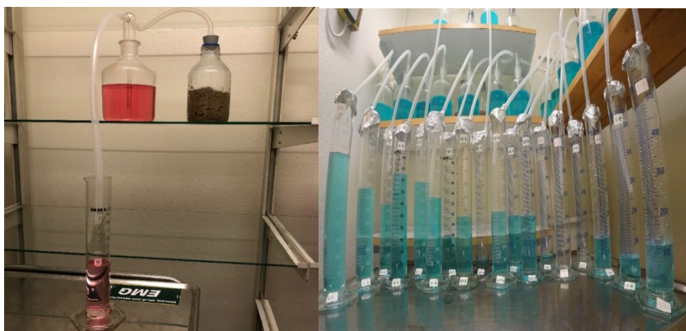
Figure 4. Gas Washing Bottle Setup. Total gas production with gas washing bottle (left) and with different concentrations of added bark extract over time (right). N=3 for each concentration. Amounts of depressed water was recorded/10 min with a camera.
