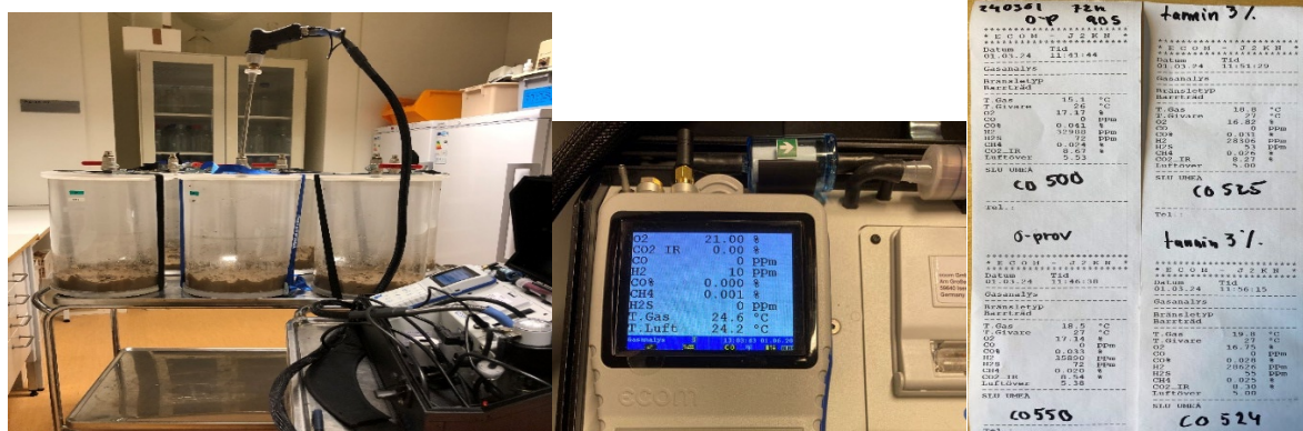
Figure 5. Experimental setup. Cylinders with pulp and the measuring probe (left), and data output (right).
