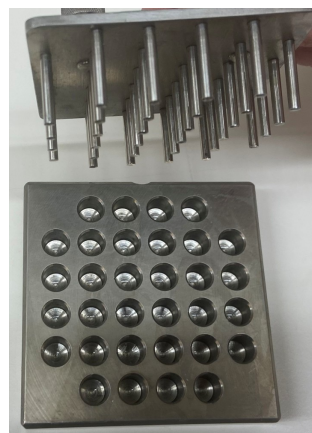
Figure 7. Illustration of the agar dilution method used for antimicrobial testing of spruce bark extract. The lowest concentration of spruce bark extract in the agar plates are determined for each tested bacterial strain, noted as MIC values.
