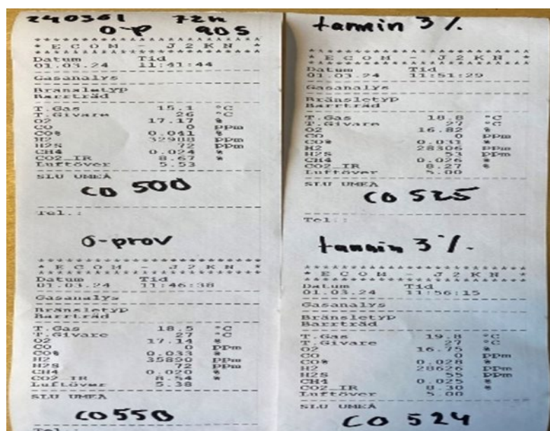
Figure 20. Gas concentration readout from ECOM analyser showing levels of CO 2 , H 2 , and other gases.
