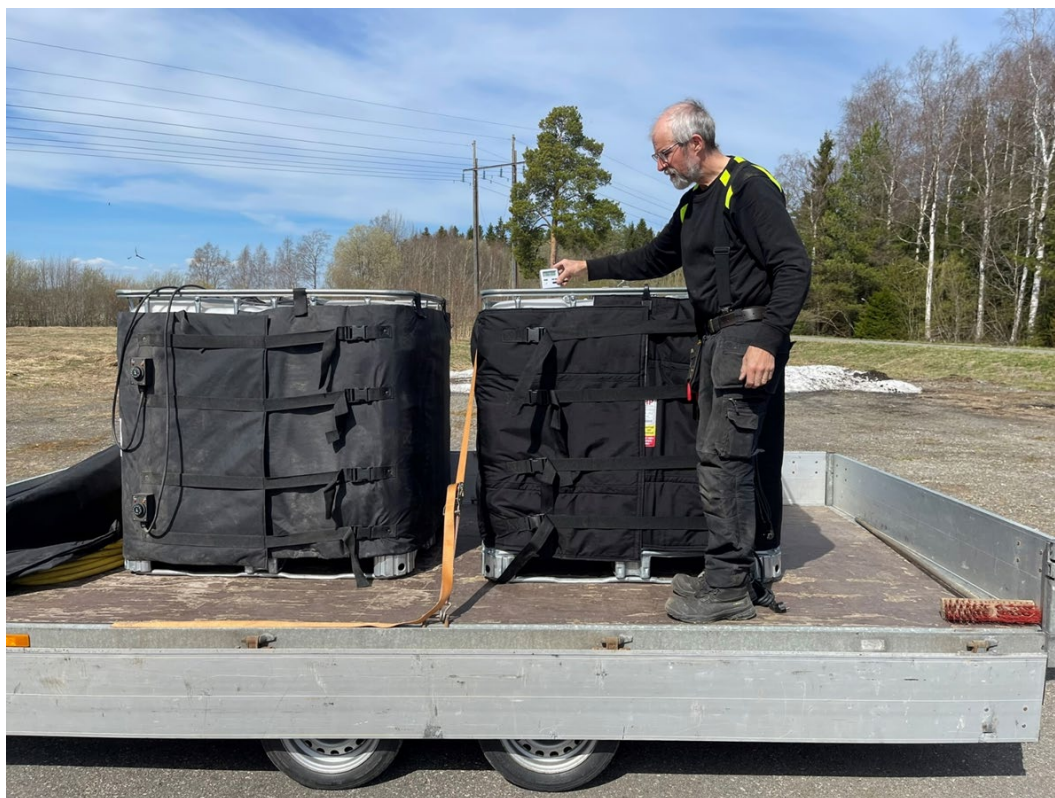
Figure 8. Recycled pulp in 1 m 3 containers with heaters to control the temperature during transport from the paper mill to the SLU pilot facilities.
