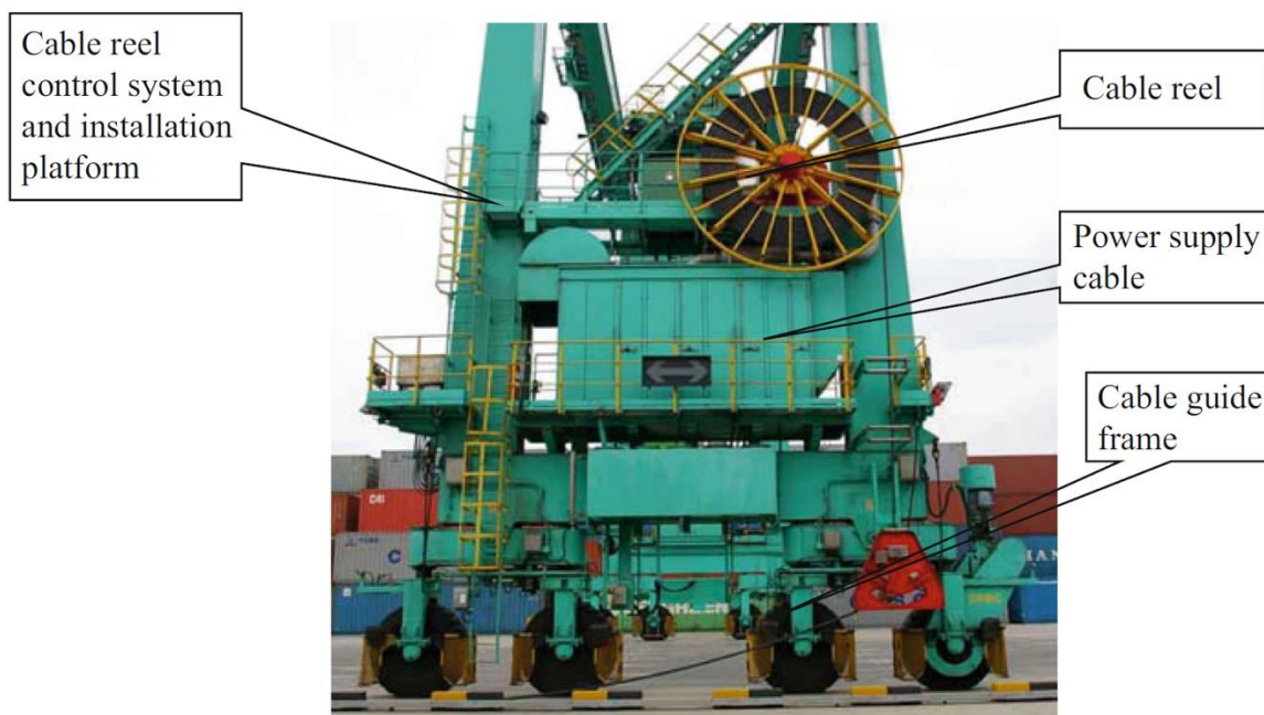
Fig. 12. Composition I of RTG power supply system with mains power supply[Handbook of Port Machinery, 2024]
