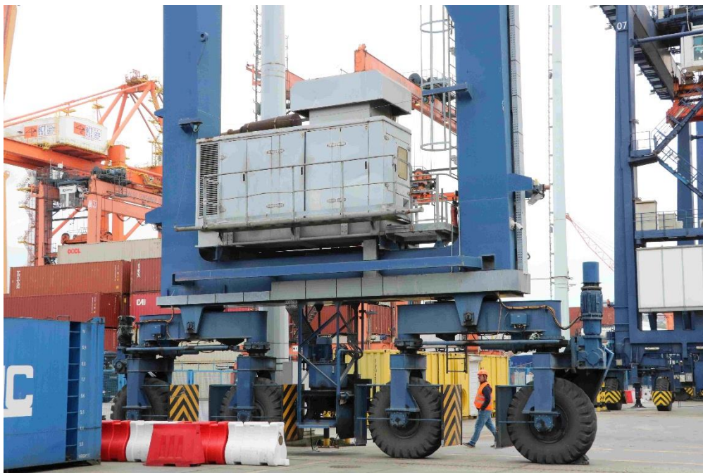
Fig. 26. Diesel generator unit in the RTG crane, which will be removed during the conversion. In its place, new electrical equipment will be installed
