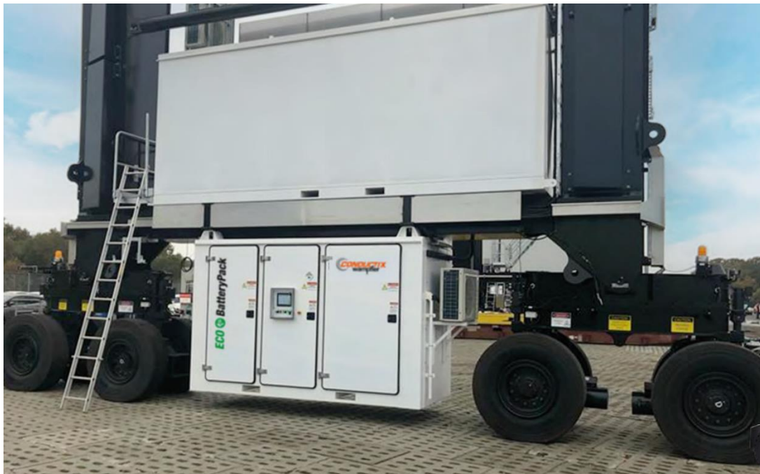
Fig. 18. Battery system in RTG crane [Conductix wampfler information materials]
