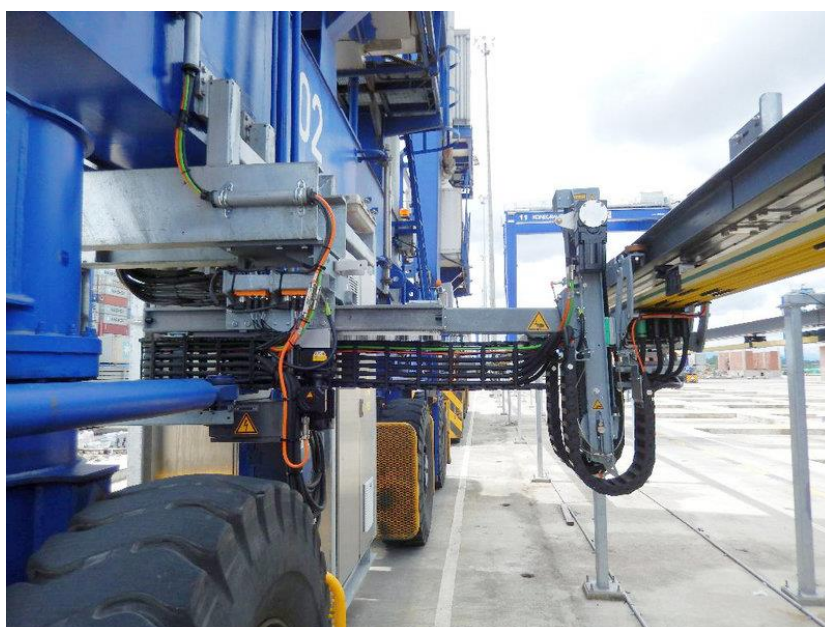
Fig. 17 .Example of Conductor Bar RTG supply system [Conductix wampfler information materials]
