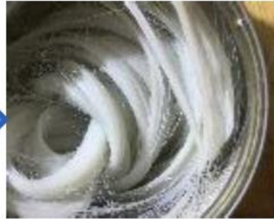
Fiber glass inside crusher
