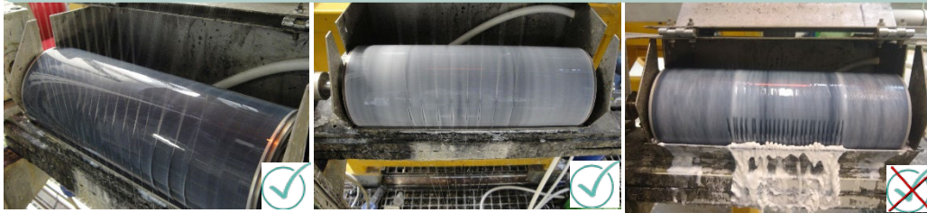
Homogeneous wetting of the sizing roll
