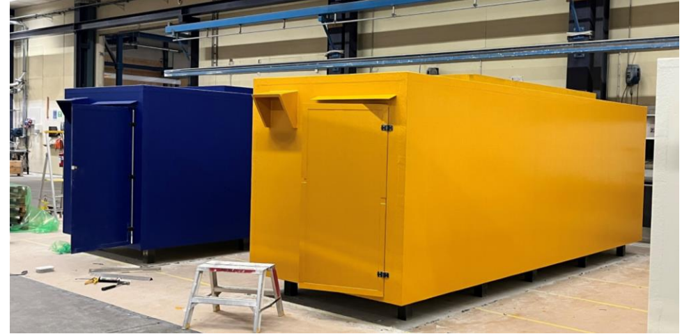
Glass fibre/PET/polyester Tank for road salt Special purpose house
