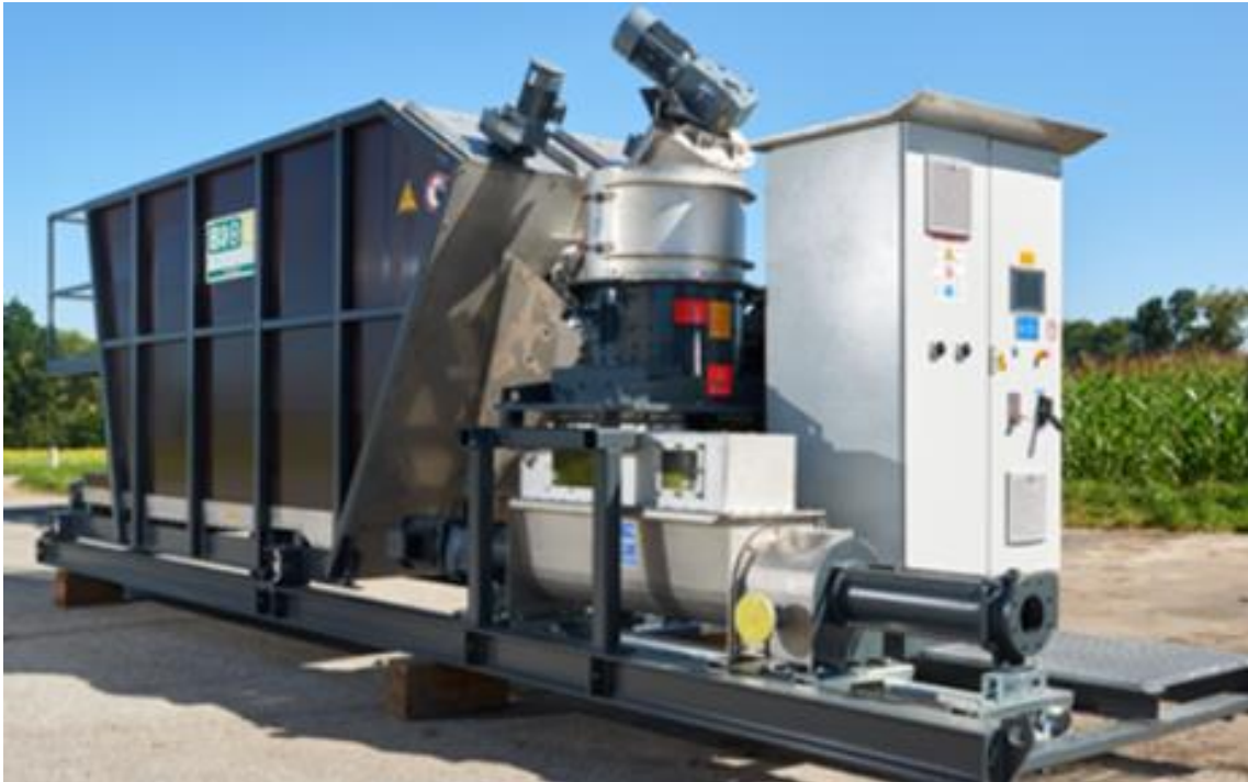
Figure 8: Substrate pretreatment unit with impact crusher system (Example: BIOG, Austria)
