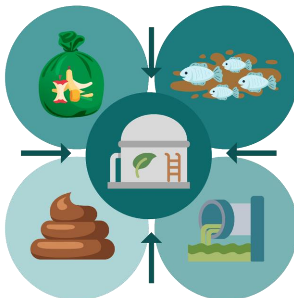
Sources for bio waste that can be anaerobically digested to produce biogas and biofertilizer.
