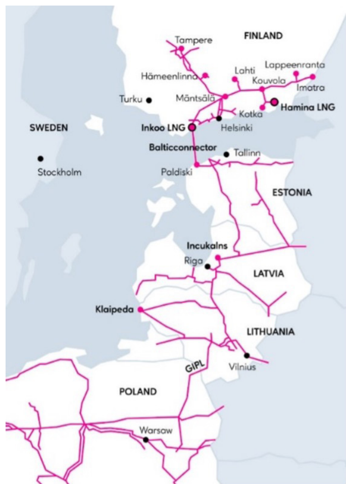
Figure 7. Gas grid in the Baltic Sea area integrated by the Baltic connector and the GIPL. 35
