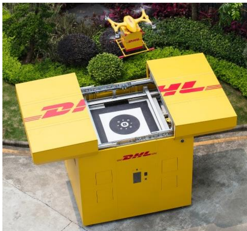
Figure 19: Medium scale landing pad by DHL (DHL Drone-in-a-Box System)
