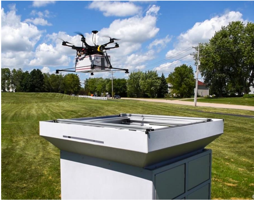
Figure 21: Medium scale landing pad by Valqari (Valqari)
