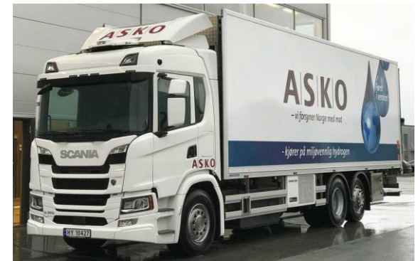
Scania Hydrogen Fuel Cell Medium distance Approx. 500 km. range
