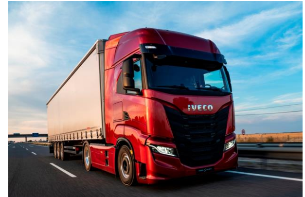
IVECO S-Way Hydrogen Long-distance 400 kW, 1800 Nm Range approx. 800 km 700 bar (?)
