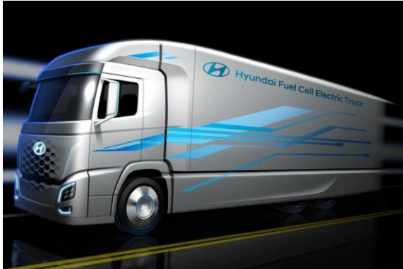
Hyundai Xcient Fuel Cell Medium distance 350 kW, 3400 Nm of torque. 8.2 kg of hydrogen H35 per 100 km Range approx. 400 km. 350 bar
