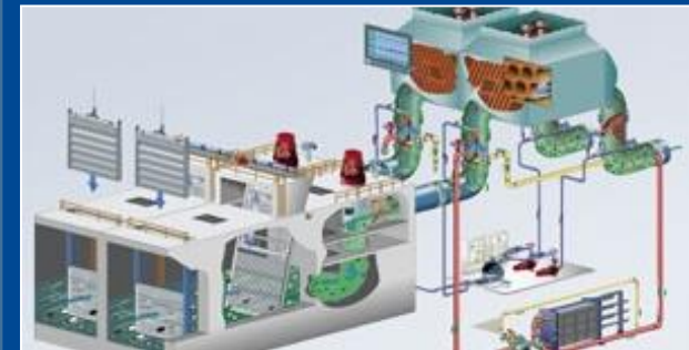
power plant – once-through cooling
