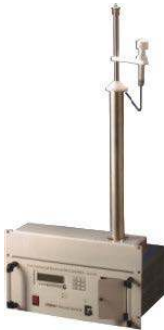
Figure 3.5. Grimm Environmental Dust Monitor, model 180.
