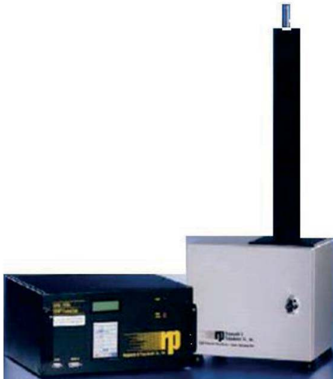
Figure 3.2. Thermo Scientific Ambient Particulate Monitor, TEOM 1400ab
