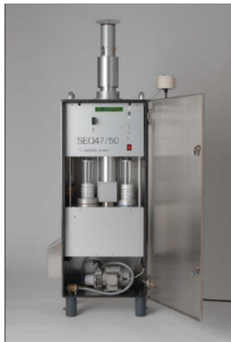
Figure 3.1a. Sequential reference sampler Leckel SEQ 47/50.
