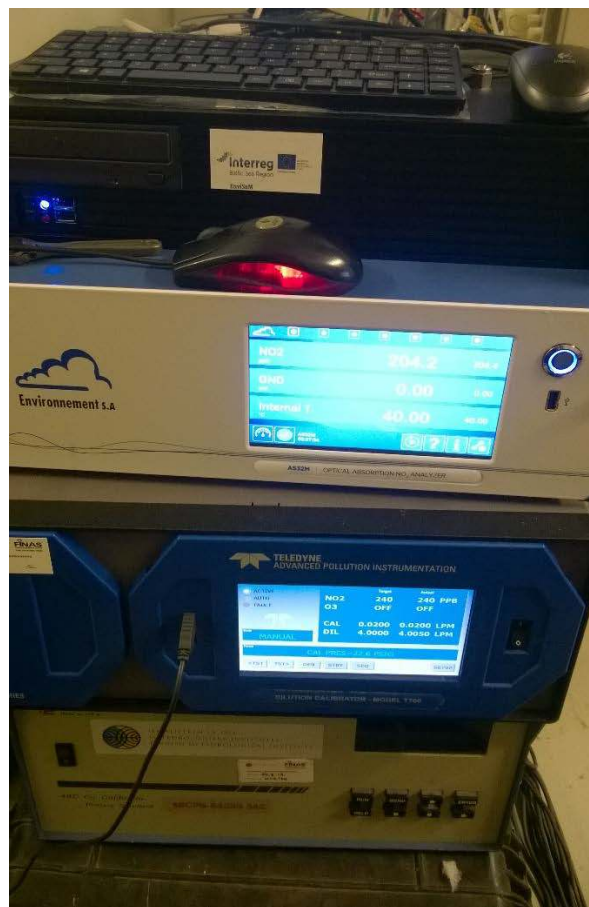
Figure 3.6. Calibration facility of FMI used for calibration of the gaseous air quality analyzers at pilot cities. The lowest unit from the bottom is the ozone calibrator, the second lowest is the gas dilutor for preparation of calibration concentrations for SO 2 , NO, NO 2 , and CO gases. The third equipment is the NO 2 analyzer and on the top is the data acquisition system.
