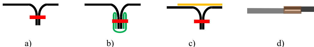
Figure 7.3. Seam types in CPC suits: a) stitched seam; b) bound seam; c) stitched and taped seam; d) welded seam [128]
