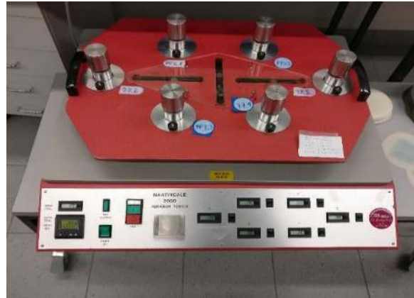
Figure 6.11. Martindale test machine with 6 specimens with pressure of 12kPa
