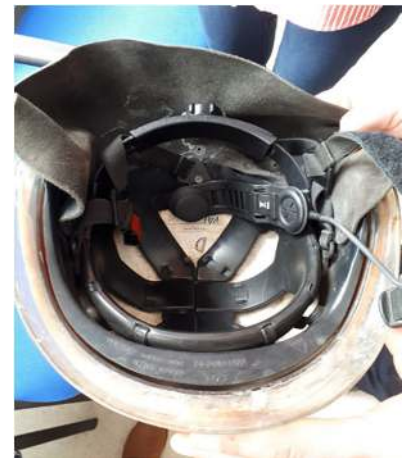
Figure 7.16. The moment of testing and helmet with integrated earpiece – bone microphone
