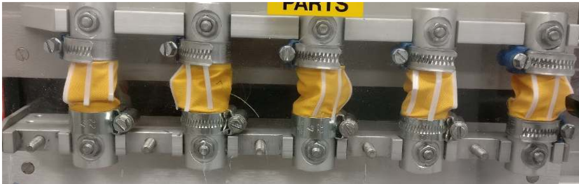
Figure 6.2. Flexing test of standard PLA
