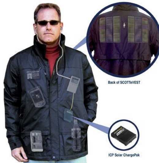
Figure 4.7. Jacket equipped with solar panels enabling recharging of the battery via the USB port
