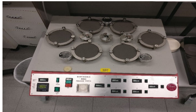
Figure 6.9. Sandpaper 1600 grits are mounted to abradant holder with foam underneath
