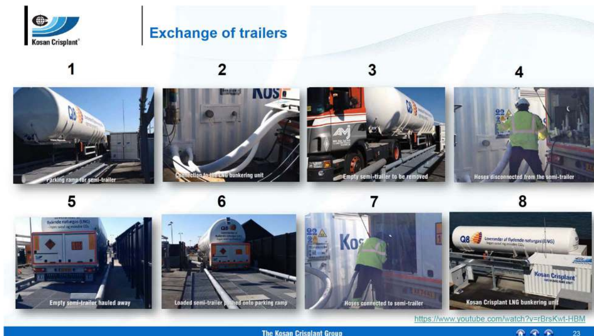
Fig. 4.12. Slide from the presentation of Frej Olsen from Kosan Crisplant on the LNG bunkering infrastructure that has been built for the Samsø ferry.
