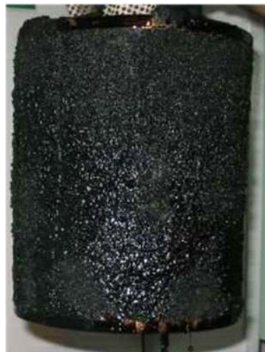
Figure 1.10 Heavily stained and blocked fuel filter of the fuel transfer pump.
