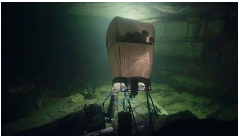
An example of a habitat, used in Plura, Norway by cave divers.
