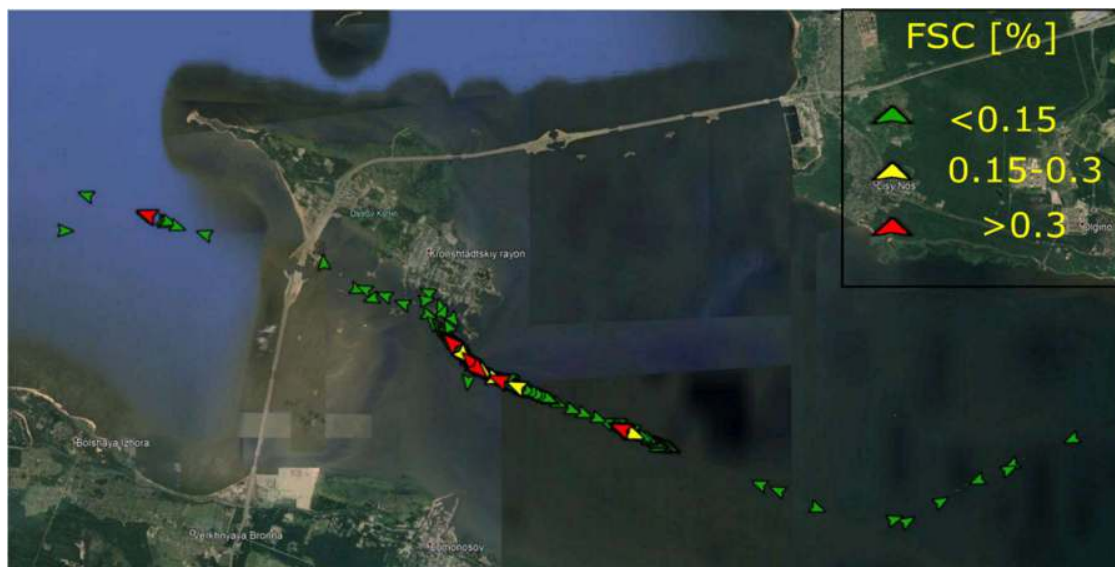
Figure 1.13 Shipborne Measurements of the Fuel Sulphur Content of individual ships in Neva bay, outside St. Petersburg. The limit for detected non-compliance is here 0.15%, taking into account the measurements error.
