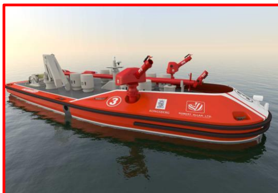
Unmanned and remotely operated fireboat
