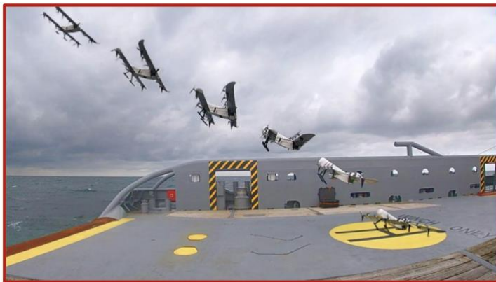
A hydrogen-powered drone capable of vertical take-off and landing whilst also being able to fly horizontally efficiently for several hours, developed by the TU Delft, together with the Royal Netherlands Navy and the Netherlands Coastguard.
