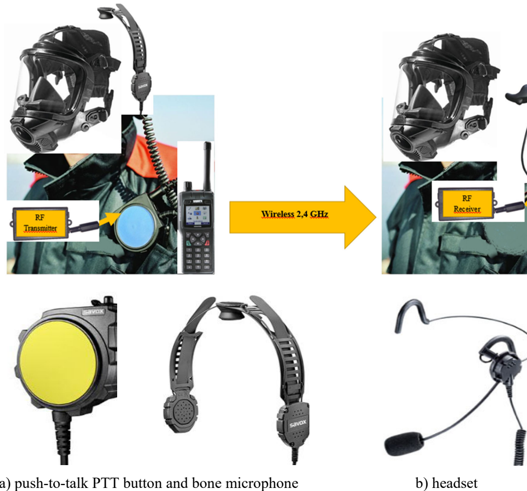
Figure 7.10. Additional devices for free hand communication inside the encapsulated CPC suit:
