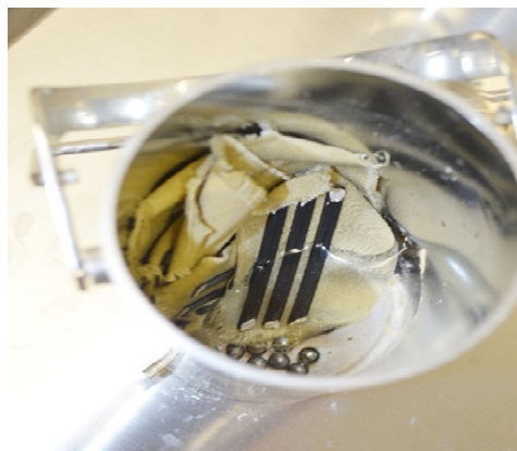
Figure 15. Samples of printed graphene PLA on fabric F2 in washing vessel
