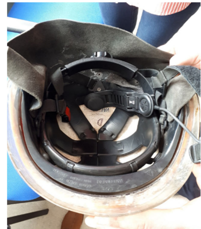
Figure 7.16. The moment of testing and helmet with integrated earpiece – bone microphone
