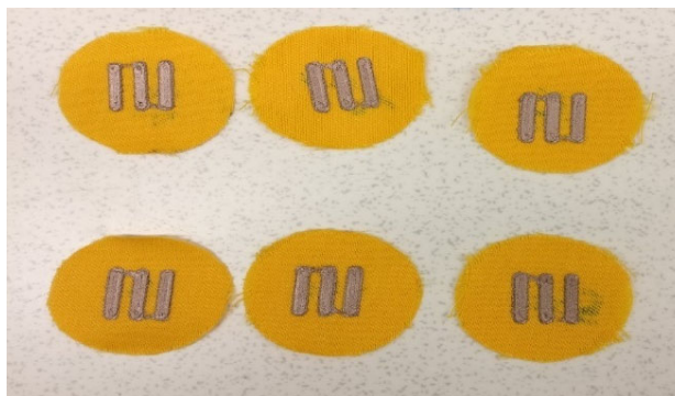
Figure 6.8. Cut sample of copper PLA on fabric F1, each sample have diameter of 30mm.
