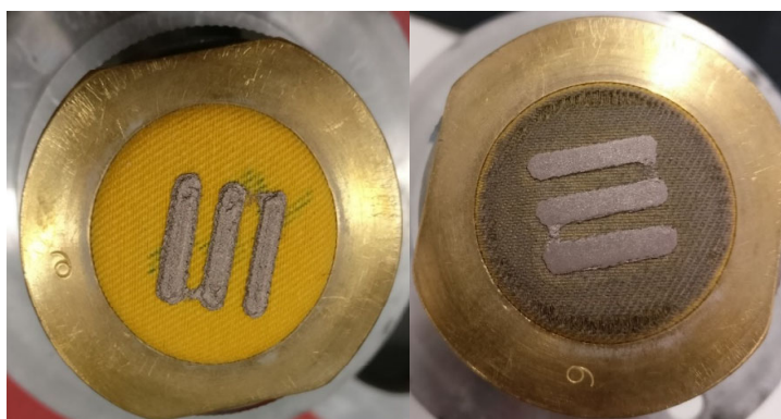
Figure 6.12. Initial specimen and after breakdown specimen (after 13000 rubs) of cooper PLA sample on fabric F1
