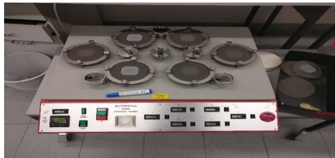
Figure 6.10. Abradant is cleaned by vacuum cleaner after each intervals (2000rubs)
