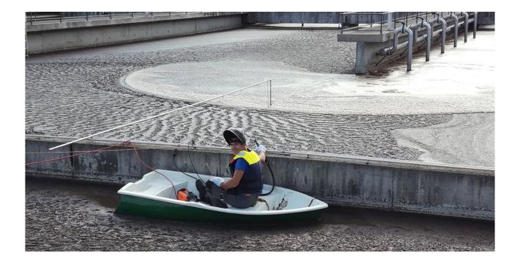
ammonia concentration directly in the active sludge. This is important step in choosing correct oxygen setpoint in the aeration tanks for nitrification. Before the installation of the new analyzer, oxygen setpoints were regulated according to ammonia concentration in the wastewater after secondary clarifiers. It resulted in process control time lag of ~6 hours.
