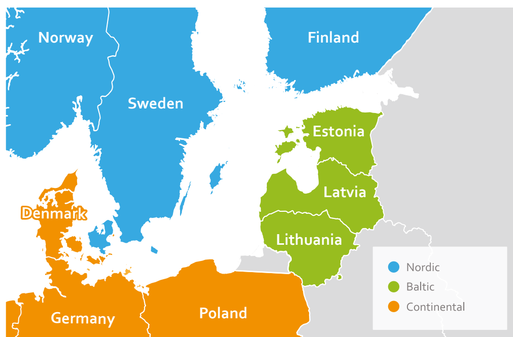
Figure 4. Synchronous grids in Europe.
